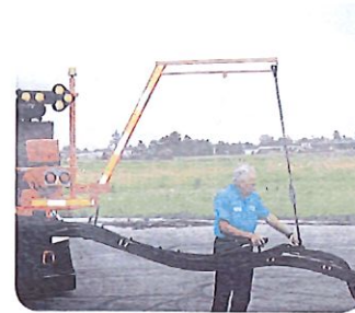
Balanced hose carrier relieves operator of any weight while providing a full range of motion.
